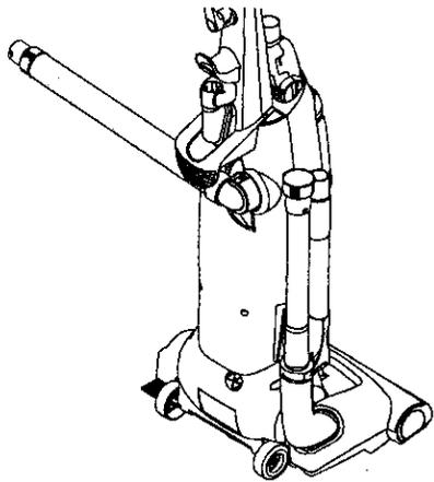
Plug in the vacuum cleaner and turn it on. Stretch the hose to maximum length and then allow the hose to return to its storage length.
